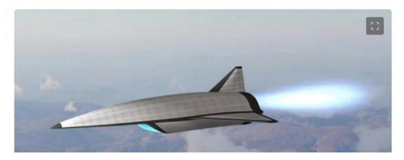
"The Mayhem system will use a scramjet engine to generate thrust, propelling the vehicle across long distances at speeds greater than Mach 5," Leidos said in a release.
